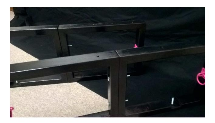
Put the two wooden cross pieces into the cut outs and loosely fit the washers and nuts
