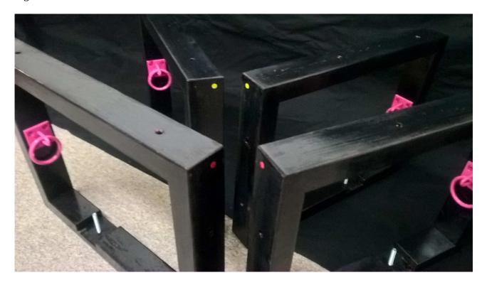
Put the short bolts in the holes of the cut-outs Put the legs together with the same coloured dots against each other.
