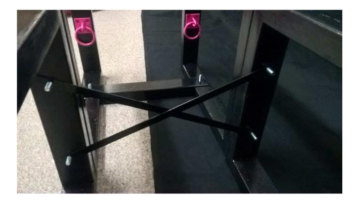
Fit the knee pad, it will only fit into one set of holes. Again loosely fit the washers and nuts
