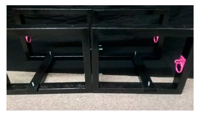
Place the metal cross pieces with 4 long bolts as shown. Again loosely fit the washers and nuts
